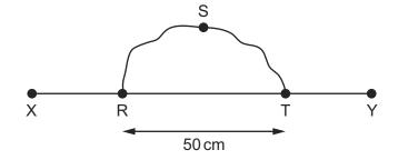
Each wire is 100 cm long with a resistance per unit length of  $10 \Omega m^{-1}$ .
