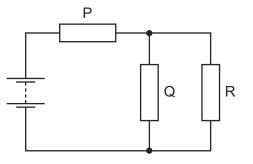
The battery, of negligible internal resistance, supplies a total power of 12W.
