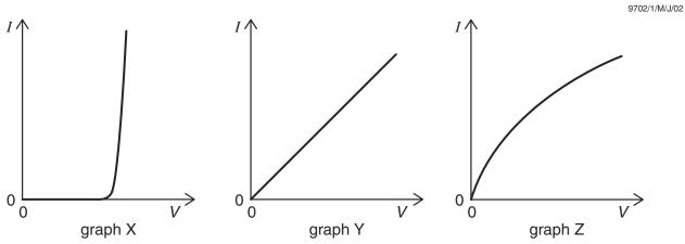
The three circuit elements are a metal wire at constant temperature, a semiconductor diode and a filament lamp.
