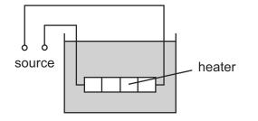
The heater has a resistance of  $3.0 \Omega$ . The voltage source has an e.m.f. of 12 V and an internal resistance of  $1.0 \Omega$ .
