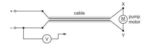
The motor does not work so, to find the fault, the negative terminal of a voltmeter is connected to the negative terminal of the power supply and its other end is connected in turn to terminals X and Y at the motor.
