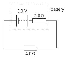
The battery is connected to a load of  $4.0 \Omega$ .
