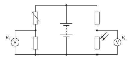
The readings on  $V_T$  and  $V_L$  are both high.
