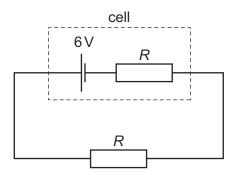
Power *P* is dissipated by the external resistor.
