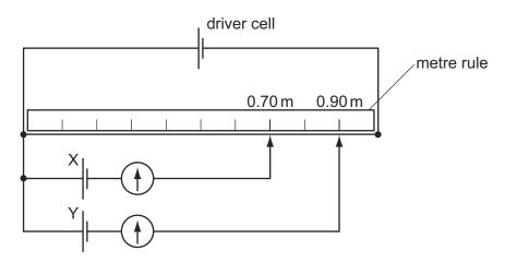
The balance points for cells X and Y are 0.70 m and 0.90 m respectively.
