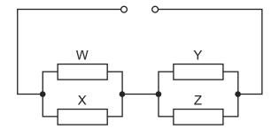
How will the powers to the resistors change when resistor W is removed?
