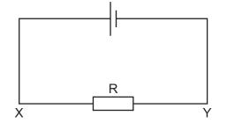
What is the rate of flow and the direction of flow of electrons through the resistor R?
