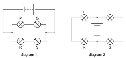
The four lamps and the battery are then connected as shown in diagram 2.
