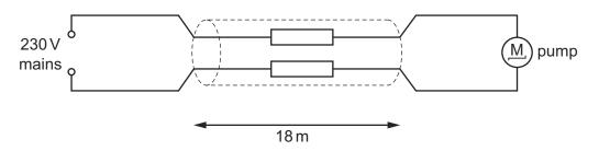
The performance of the pump is acceptable if the potential difference (p.d.) across it is at least 218 V. The current through it is then 0.83 A.
