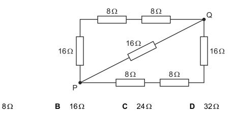
**35** The combined resistance  $R_T$  of two resistors of resistances  $R_1$  and  $R_2$  connected in parallel is given by the formula shown. 9702/11/O/N/14
