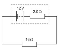
What is the power dissipated in the  $13\Omega$  resistor?
