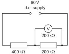
What is the reading on a voltmeter, also of resistance 200 k $\Omega$ , when connected across the 200 k $\Omega$  resistor as shown in the diagram?
