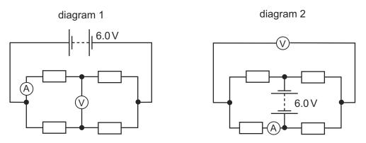
The resistors and meters are reconnected to the supply as shown in diagram 2.
