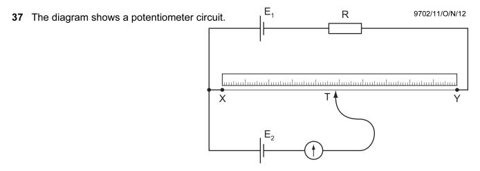
The contact T is placed on the wire and moved along the wire until the galvanometer reading is zero. The length XT is then noted.
