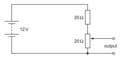
The fixed resistor and the potentiometer each have resistance  $20 \Omega$ . The circuit is designed to provide a variable output voltage.
