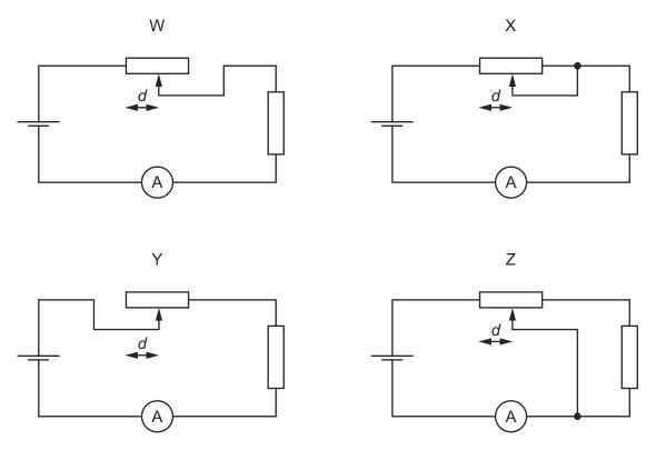
The distance d between the sliding contact and a particular end of the potentiometer is varied. The current measured is then plotted against the distance d.
