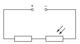
When the LDR is in the dark, the fixed resistor and the LDR have the same value of resistance.
