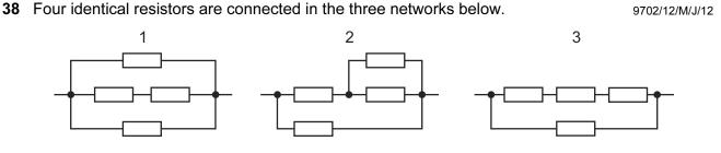
Which arrangement has the highest total resistance and which has the lowest?
