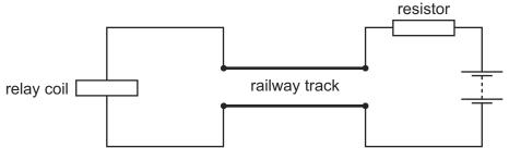
With no train present, there is a current in the relay coil which operates a switch to turn on a light.
