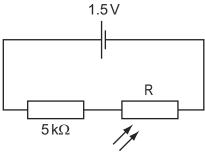
The light-dependent resistor is illuminated (in an otherwise dark room) by a flashing light.
