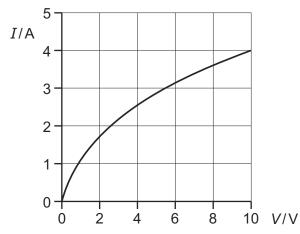
Since the graph is not a straight line, the resistance of the lamp varies with V
